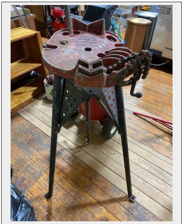
**Description**Ridgid tristand 1/8 to 6. Heavy duty pipe bending, cutting and threading table
